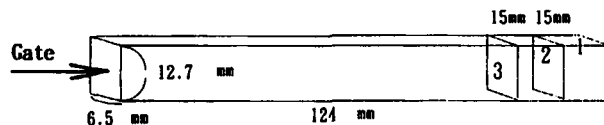
Figure 1 Schematic illustration of the sections taken from the injection-molded bars. (1) Skin, (2) middle, (3) core.
